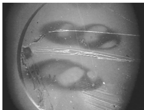
FIG. 6. Optical image of an electron-irradiated CaF 2 sample after several localized bleaching treatments at 157 nm. The dark ovals were produced by electron irradiation. The clear spots in the ovals were produced by various 157 nm treatments.
