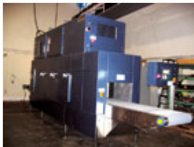
Engineers from England's Strayfield Ltd. installed this RF unit at Diamond Foods to test radio frequencies as an alternative to chemical fumigants in post-harvest nuts. Source: Washington State University.
